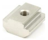
These nuts are the fastest and easiest way to bolt things on to your T-Slot structure. They slide into the namesake slot and provide a mounting point that you can bolt external parts onto with M5 bolts.
