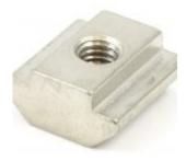
These nuts are the fastest and easiest way to bolt things on to your T-Slot structure. They slide into the namesake slot and provide a mounting point that you can bolt external parts onto with M6 bolts.
