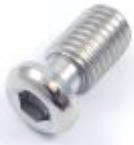
The most basic way to attach 2 extrusions at right angles is to simply bolt them together like you would a 2x4. These screw connectors require that you tap the center hole in one extrusion with an M14x2 tap and access for an allen key drilled in the opposite extrusion so the bolt can be tightened.
