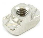
The T-nuts provide an option for a mounting point that can be installed in the middle of an extrusion without having to slide the nut all the way in from the end. This allows for faster installation as well as installation after the structure has been fully constructed, it does require a bit of finesse to install properly though. Have a look at the T-Slot primer in the resources section for more information on installation. These nuts are suitable for use with M6 bolts.
