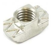
The T-nuts provide an option for a mounting point that can be installed in the middle of an extrusion without having to slide the nut all the way in from the end. This allows for faster installation as well as installation after the structure has been fully constructed, it does require a bit of finesse to install properly though. Have a look at the T-Slot primer in the resources section for more information on installation. These nuts are suitable for use with M8 bolts.
