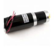
The DCM4002 is a 24 volt motor, generating 45 kg-cm of torque with a top speed of 182 RPM. For more details on the torque and speed characteristics of the motor, see the torque curves document on the Resources tab.
