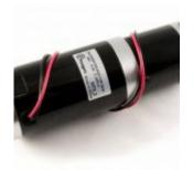
The 3273 is a 24 volt gear motor, generating 82.6 Kg-cm of torque at 33 RPM. It's a large motor that provides an amazing amount of torque.
