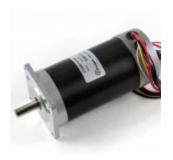
The DCM4112 is a 24 volt brushless DC motor, generating 4.9 Kg-cm of torque at 4000 RPM.
