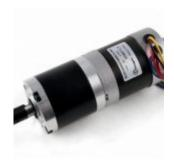
The DCM4111 is a 24 volt brushless DC motor, generating 210 Kg-cm of torque at 41 RPM. The shaft is equipped with a 4mm key to improve coupling.
