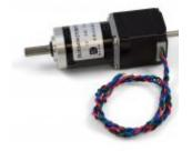
This NEMA-11 motor has an integrated Planetary gearbox with a  $26^{103}/_{121}$ :1 ratio. It comes with the rear shaft exposed, so you can mount an encoder or shaft coupler. See the "Compatible Products" tab for a complete list of attachments.
