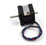
This NEMA-17 motor generates 3.6 Kg-cm of holding torque at 1.7 Amps. It comes with the rear shaft exposed, so you can mount an encoder or shaft coupler. See the "Compatible Products" tab for a complete list of attachments.
