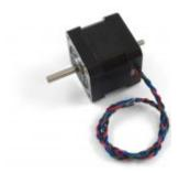
This NEMA-17 motor generates 3.6 Kg-cm of holding torque at 1.7 Amps. It comes with the rear shaft exposed, so you can mount an encoder or shaft coupler. See the hardware section for a list of compatible accessories.
