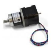
This NEMA-17 motor has an integrated Planetary gearbox with a 26  $^{103}/_{121}$ :1 ratio. It comes with the rear shaft exposed, so you can mount an encoder or shaft coupler. See the "Compatible Products" tab for a complete list of attachments.
