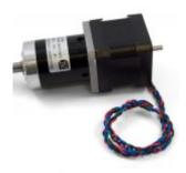
This NEMA-17 motor has an integrated Planetary gearbox with a  $50^{4397}/_{4913}$ :1 ratio. It comes with the rear shaft exposed, so you can mount an encoder or shaft coupler. See the "Compatible Products" tab for a complete list of attachments.
