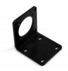
This coated steel mounting bracket provides a simple means of attaching a NEMA-23 sized motor to a flat surface. It has two sets of mounting holes, so it can be attached to 56mm planetary gearboxes or mounted directly to the motor. For a list of compatible motors, see the "Compatible Products" tab.
