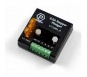
If you're looking for a compact solution for controlling a medium-sized stepper motor, the STC1001 is an affordable and convenient option. You can control the position, velocity, and acceleration of the motor by sending commands from your program. This Phidget connects to a VINT Hub; for a list of options see the "Compatible Products" tab.
