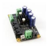
**Note:** This revision of the 1065 comes with a built-in heatsink for the driver chip to prevent it from overheating.
