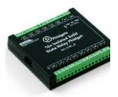
For applications that require a ton of outputs, this module is the one you're looking for. With sixteen PWM-enabled relay outputs, not only can it handle orindary logic-level devices at 3.3V or 5V, but it can also be used to control devices of up to 30V volts and 8 amps. LED strips, DC motors, power relays, fans and other small circuits are all common loads for this type of output. The REL1101 connects to a port on a **VINT Hub**. See the "Comaptible Products" tab for a list of hubs.
