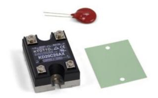
This SSR comes with a heat transfer pad and a TMOV20RP200E varistor. Use the heat transfer pad whenever mounting the SSR on a heat sink or metal surface. If you're switching a load at 120V or less, you can put the varistor across the load terminals in parallel with the rest of the load circuit in order to protect your relay from voltage spikes. If you're switching a load higher than 120V, do not use the varistor. For more information, see the <u>Solid State Relay Primer</u>.
