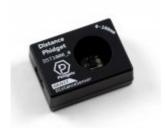
Do you need a sensor that can measure short distances or detect the motion of objects passing by? This Phidget uses infrared light and a time-of-flight calculation to determine how far away an object is. It can report the distance of the object it's pointed at as often as every 10 milliseconds, and will throw a saturation event when the distance exceeds the sensor's maximum range. Since infrared light is what it uses for the measurement, highly reflective objects will be easier to measure.
