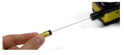
When the wire is pulled out, the sensor produces a quadrature signal to describe the length of wire exposed. The reel is spring loaded, so it will retract when there is no tension in the wire. Multiple draw wire sensors could be used to track the position in more than one dimension.
