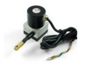
In complex mechanical systems, it is often very difficult to accurately measure the movement of a single part, particularly if it has several degrees of freedom. The draw wire encoder is a versatile solution to this very problem; it can be attached to a part using an M5 screw or fastened to the end with a zip tie, and the encoder itself has a pair of M4 screw threads on the back for easy installation.
