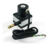
In complex mechanical systems, it is often very difficult to accurately measure the movement of a single part, particularly if it has several degrees of freedom. The draw wire encoder is a versatile solution to this very problem; it can be attached to a part using an M5 screw or fastened to the end with a zip tie, and the encoder itself has a pair of M5 screw threads on the back for easy installation.
