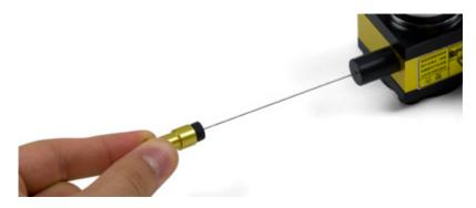
When the wire is pulled out, the sensor produces a quadrature signal to describe the length of wire exposed. The reel is spring loaded, so it will retract when there is no tension in the wire. Multiple draw wire sensors could be used to track the position in more than one dimension.
