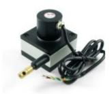
In complex mechanical systems, it is often very difficult to accurately measure the movement of a single part, particularly if it has several degrees of freedom. The draw wire encoder is a versatile solution to this very problem; it can be attached to a part using an M5 screw or fastened to the end with a zip tie, and the encoder itself has four M3 screw threads on the back for easy installation.
