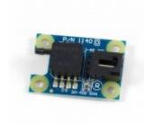
Note: The 1140\_1B is the same as the 1140\_0, except it has a different sensor that has an upward-facing port and you have the option of which size of Phidget cable to include.
