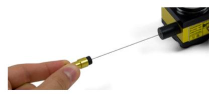
When the wire is pulled out, the sensor produces a voltage to describe the length of wire exposed. The reel is spring loaded, so it will retract when there is no tension in the wire. Multiple draw wire sensors could be used to track the position in more than one dimension.
