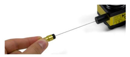
When the wire is pulled out, the sensor produces a voltage to describe the length of wire exposed. The reel is spring loaded, so it will retract when there is no tension in the wire. Multiple draw wire sensors could be used to track the position in more than one dimension.
