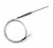
Measure -50 to 500?°C with this stainless steel class B PT1000 RTD probe. As an RTD this probe offers excellent accuracy and very low drift in comparison to what a thermocouple can offer.
