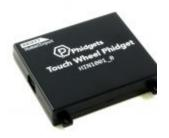
Need a user-friendly control panel for your Phidgets project? Look no further than the Touch Wheel Phidget. This user interface board uses capacitive touch technology, similar to the touchscreen on a smartphone. Capacitive touch sensors such as this can detect a touch through a piece of glass or plastic of up to 3mm thick, so you can hide this board inside an enclosure or behind a panel. The HIN1001 connects to a port on a **VINT Hub**. See the "Comaptible Products" tab for a list of hubs.
